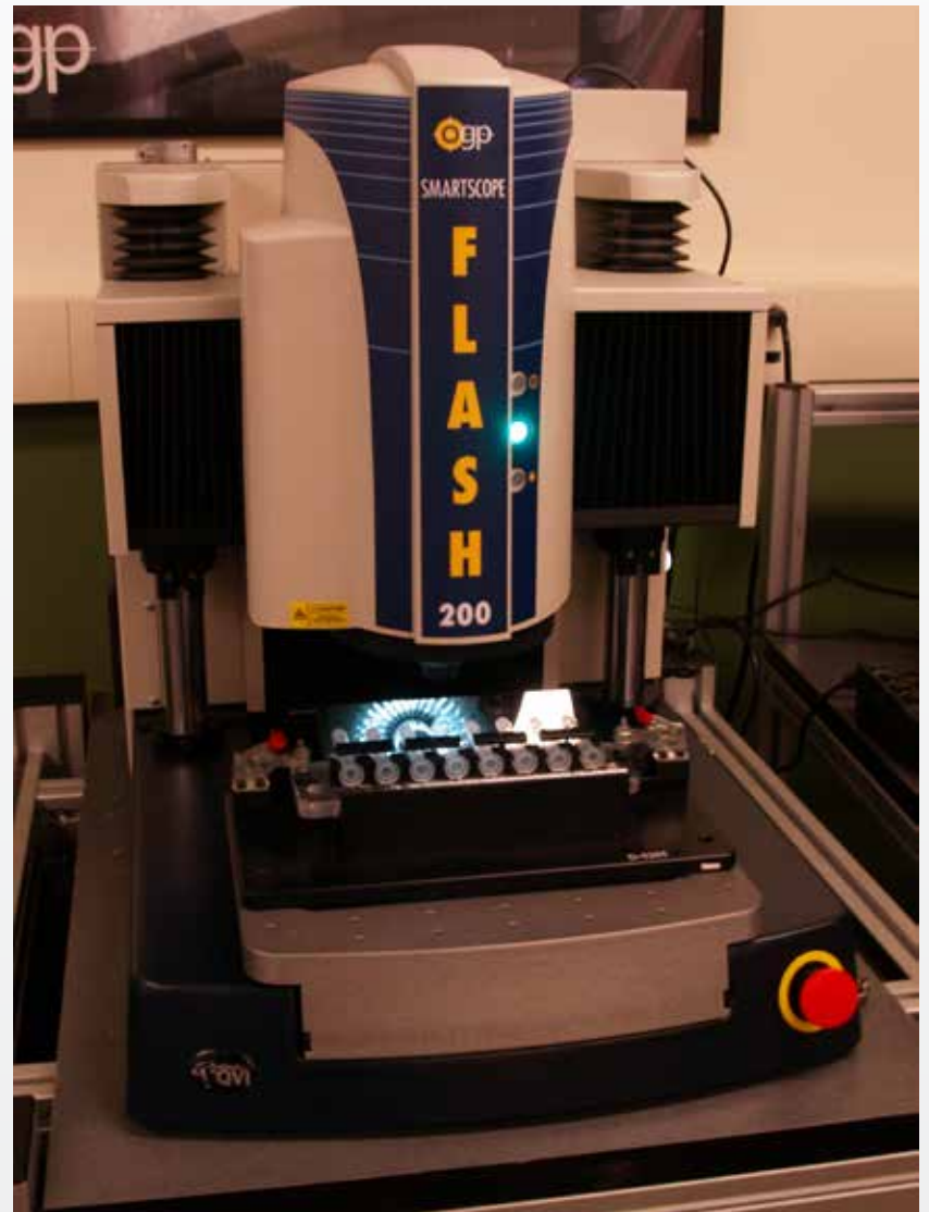
Eight syringes on a custom gang fixture.
